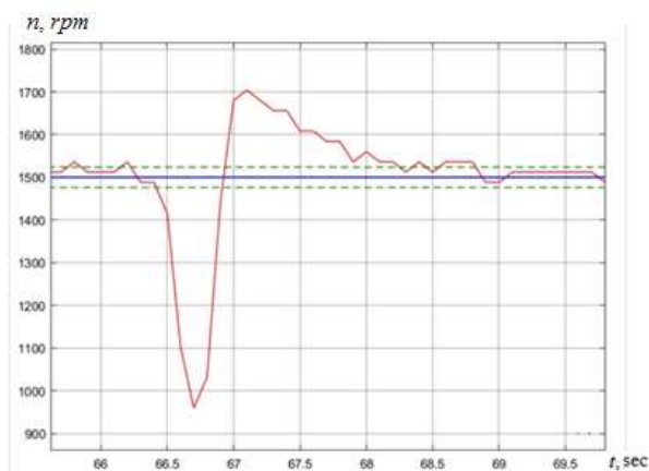
Figure 17. Response to disturbances of the closed-loop controller with coefficients K_p = 0.01 , K_i = 0.1
