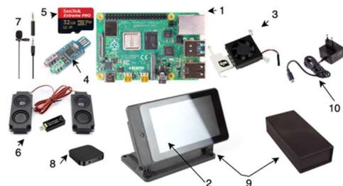
1) Raspberry Pi-4 single-board computer, 2) screen, 3) cooling system, 4) sound card, 5) storage, 6) speakers, 7) microphone, 8) audio receiver/transmitter, 9) case, 10) power supply
