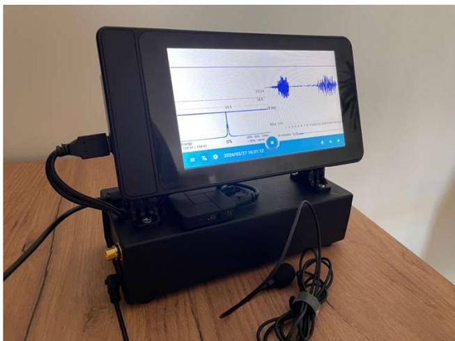
Figure 12. The device for identifying the recurrent laryngeal nerve with the function of automatic adjustment of an electrical signal.
