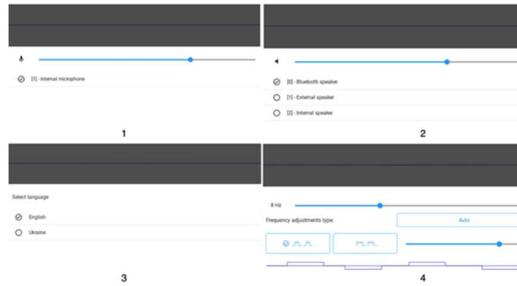
1) the microphone setting screen form; 2) the screen form for setting speakers; 3) the screen form for localization of application; 4) the screen form for setting the frequency of generation of rectangular pulses;
